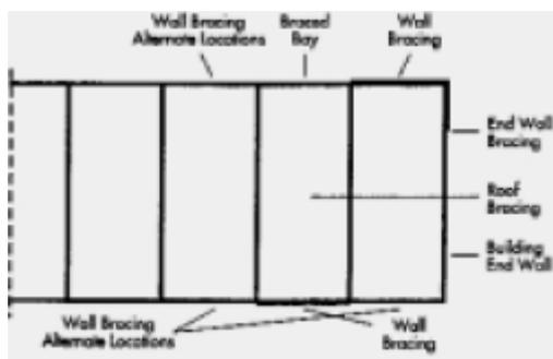
Figure A1. Building bracing location – internal bay
