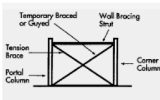
Figure A12. Wall temporary tension brace.
