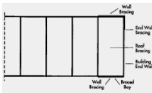
Figure A3. Building bracing location – end bay
