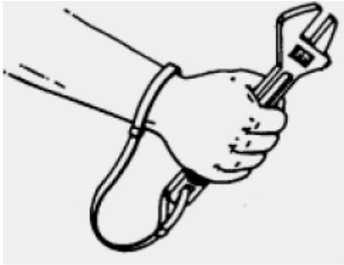
**Figure 3.** Tool attached by lanyard to wrist.
