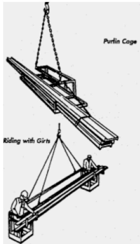
**Figure 6.** Example of purlin and girt cage/cradle
